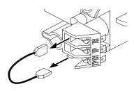
Figure 37 - Disconnecting TH to TPTH Wire
